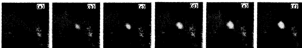
Fig. 2 CCD photos of laser trapped rubidium atoms. The light area in middle of each photo is the trapped atoms, (a) to (f) correspond a successive increase of the gradient of magnetic field. (a) 0.0005 T/cm; (b) 0.0007 T/cm; (c) 0.0009 T/cm; (d) 0.0011 T/cm; (e) 0.0014 T/cm; (f) 0.0016 T/cm
